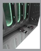
Compression tabs, shown to the left, allow the filter to snap into place, holding the filter securely against the filter gasket. The Camfil Farr Fast Frame is an air filter holding frame for built-up bank HVAC systems. The unique design allows for a convenient and simple filter replacement without sacrificing the integrity of the filter seal or compromising indoor air quality. Filter installation is quick and easy without the hassle of clips and fasteners associated with other systems.
